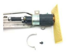
2 – loosen the OE hose clamp from the pump outlet side of the hose and remove the pump, if the OE hose is in useable condition, the other permanent clamp may be left in place. If the hose needs to be replaced, remove the second permanent clamp and remove the hose
