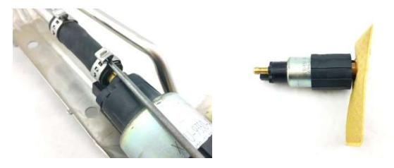
3 – remove the rubber top cap from the DW300m and reuse the pump isolator and install the new fuel sock and sock retainer
